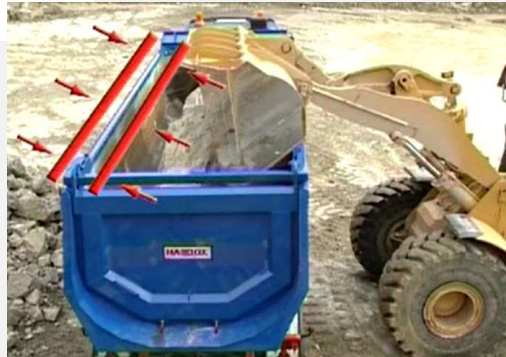
Upgrading example of Tipper Body Top Rails
