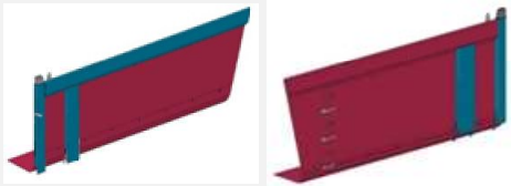
Body Sides Assembly (LH & RH side) – 3 mm thk Hardox 450 Strip - 1500 mm width
