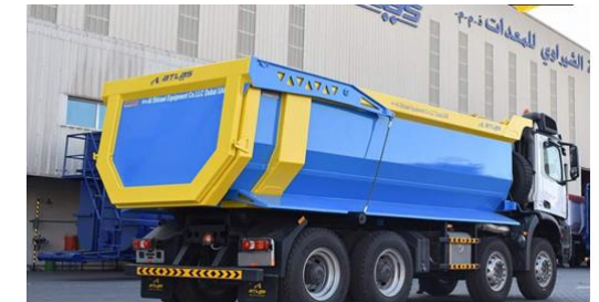
Under construction 8 mm (all) 23 cbm tipper Hardox ® 500Tuf (upgraded from Hardox ® 450) Atlas Al Shirawi, UAE
