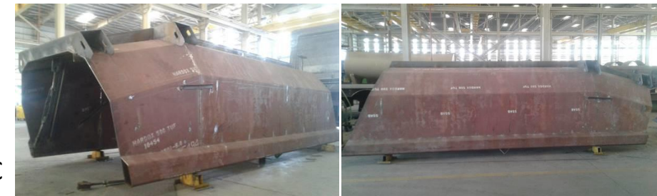
Under construction 8 mm (all) 23 cbm tipper Hardox ® 500Tuf (upgraded from Hardox ® 450) Atlas Al Shirawi, UAE
