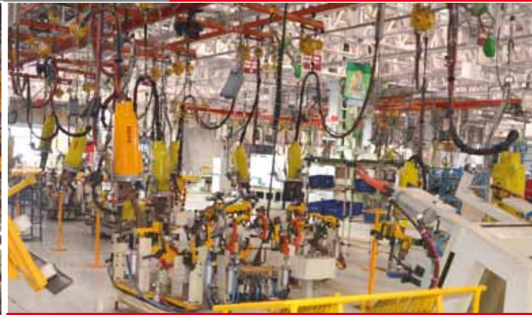
CHAKAN PLANT: The body shop has 86 assembly stages, electrified monorail system for cabin assembly, IT type weld-guns for power efficiency, robotics and advanced processes.
